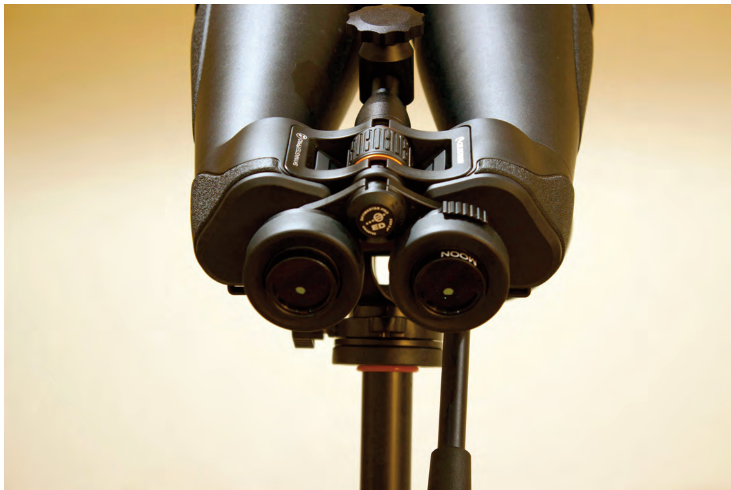
Image 21 – The eyepieces are threaded to receive 1.25-inch filters. The eyecups must be fully retracted to insert the filters, but then can be rotated out past the filters.
