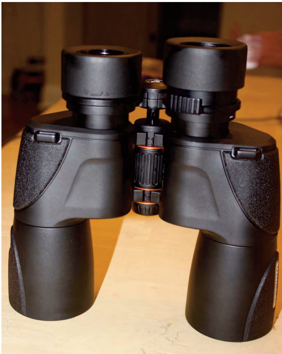
Image 3 – The eyecups on the 7x50mm binoculars rotate in and out. The one on the left is fully retracted while the one on the right is fully extended. There is a large easy to grip focusing knob. The right eyepiece has large handles to adjust it individually.
