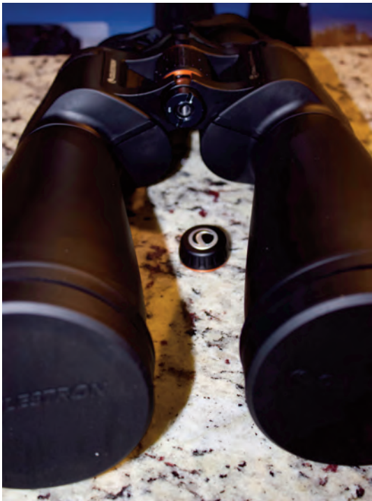
Image 9 – This view shows the large focusing knob on the 15x70mm binoculars and the cap removed for the tripod adapter connection.
