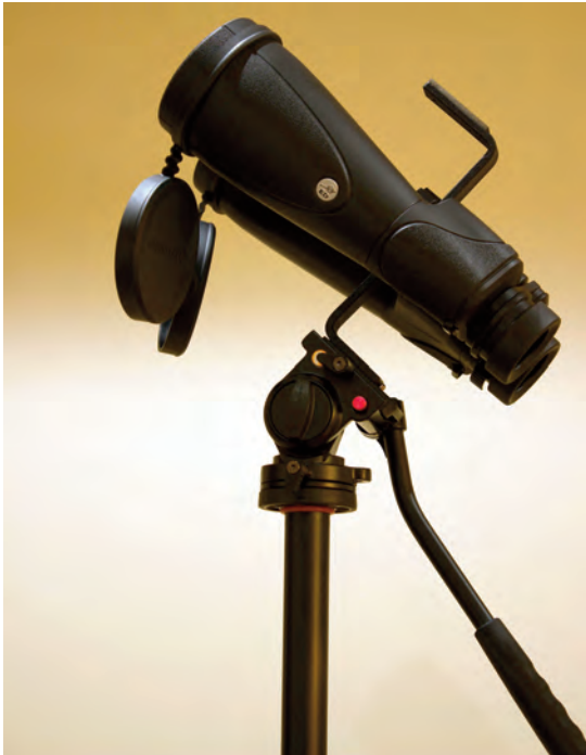
Image 10 – The author used his universal binoculars z adapter to attach the 15x70mm binoculars to a standard camera tripod. The tripod connection point is at the binoculars' center of gravity to provide perfect balance when attached this way to a tripod.
