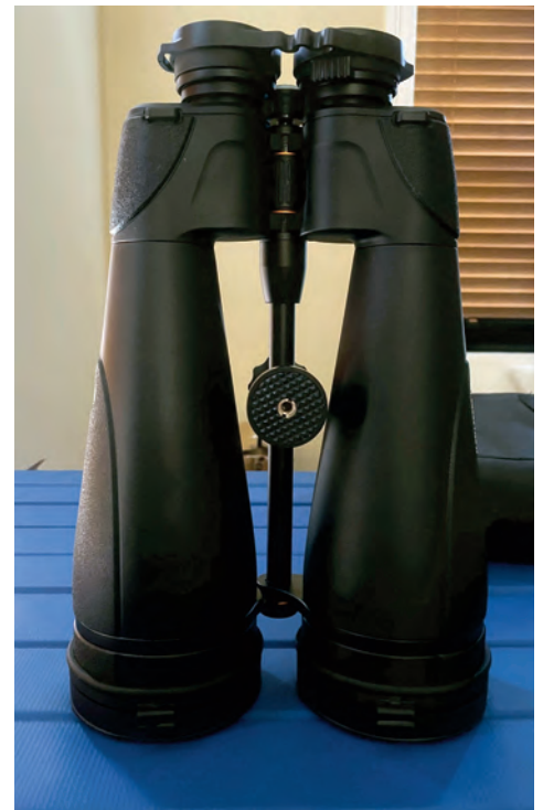
Image 17 – The 20x80mm binoculars come with a 1/4-20 threaded adapter for use on tripods. The adapter can slide up and down a shaft and locked in place for balancing.
