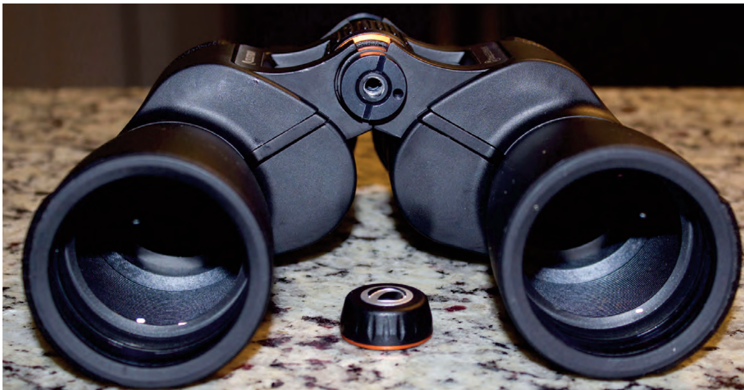
Image 4 – This view shows the objective lenses of the 7x50mm binoculars and the removable cap over the 1/4-20 threaded hole for a tripod adapter.
