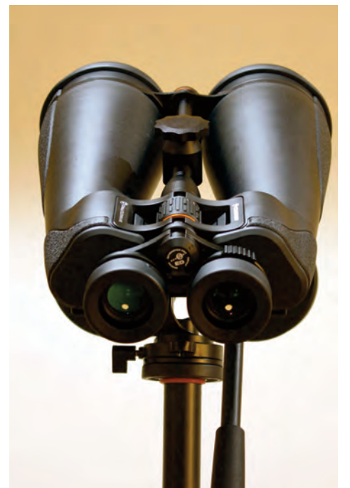
Image 18 – This view shows the hand-grip for locking down the tripod adapter in place to balance the binoculars on a tripod.
