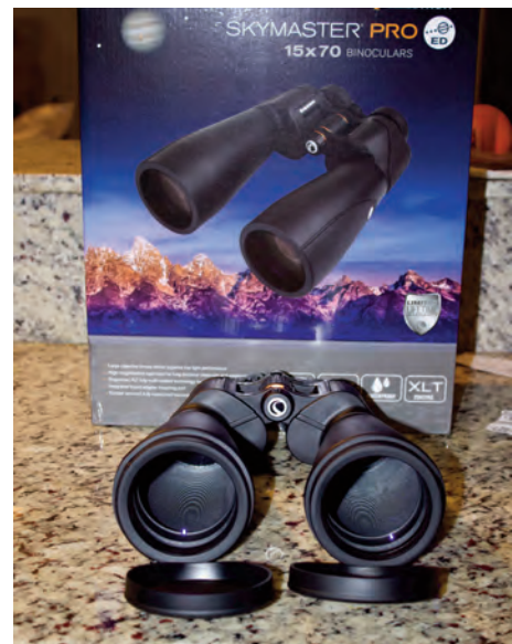
Image 8 – This view shows the objective lenses of the 15x70mm binoculars and the removable cap covering the 1/4-20 threaded hole for a tripod adapter.
